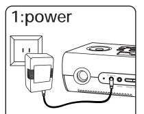
Attach AC adaptor cable to DC jack on back of the ZN9 and plug the other end into a wall socket.
